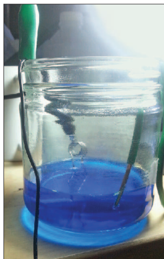
Figure 4 — Using copper electroplating techniques; you can tame Nichrome wire and give it an easily solderable copper coating. [Bennett Wilson, AF2RF, photo]
