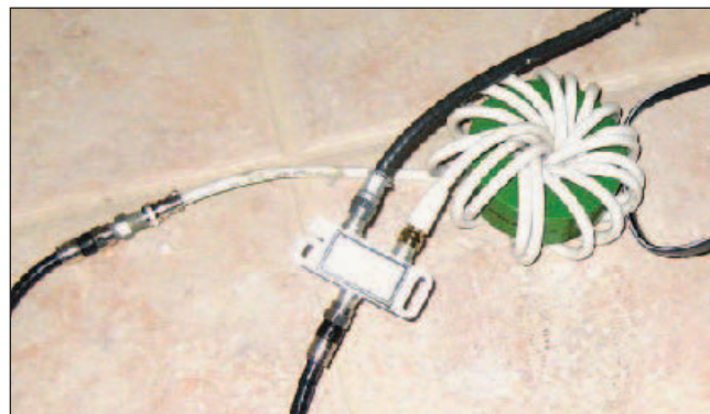
Figure 4 — A common mode choke on the coax cable. Note that an added length of coax was connected with a double female socket to provide a length of the needed turns. QST
