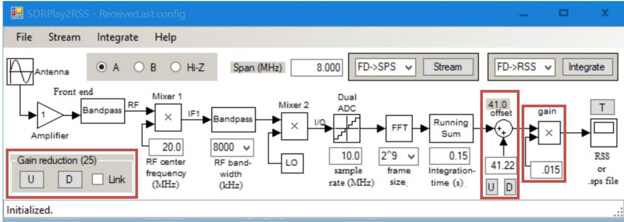
Gain reduction is applied in the RF sections of the SDRPlay RSP2 while Offset and Gain are applied after the fast Fourier transform (FFT) has been computed. The digital output of Nathan Towne’s SDRPlay2RSS is passed to Jim Sky’s Radio Sky Spectrograph (RSS).
