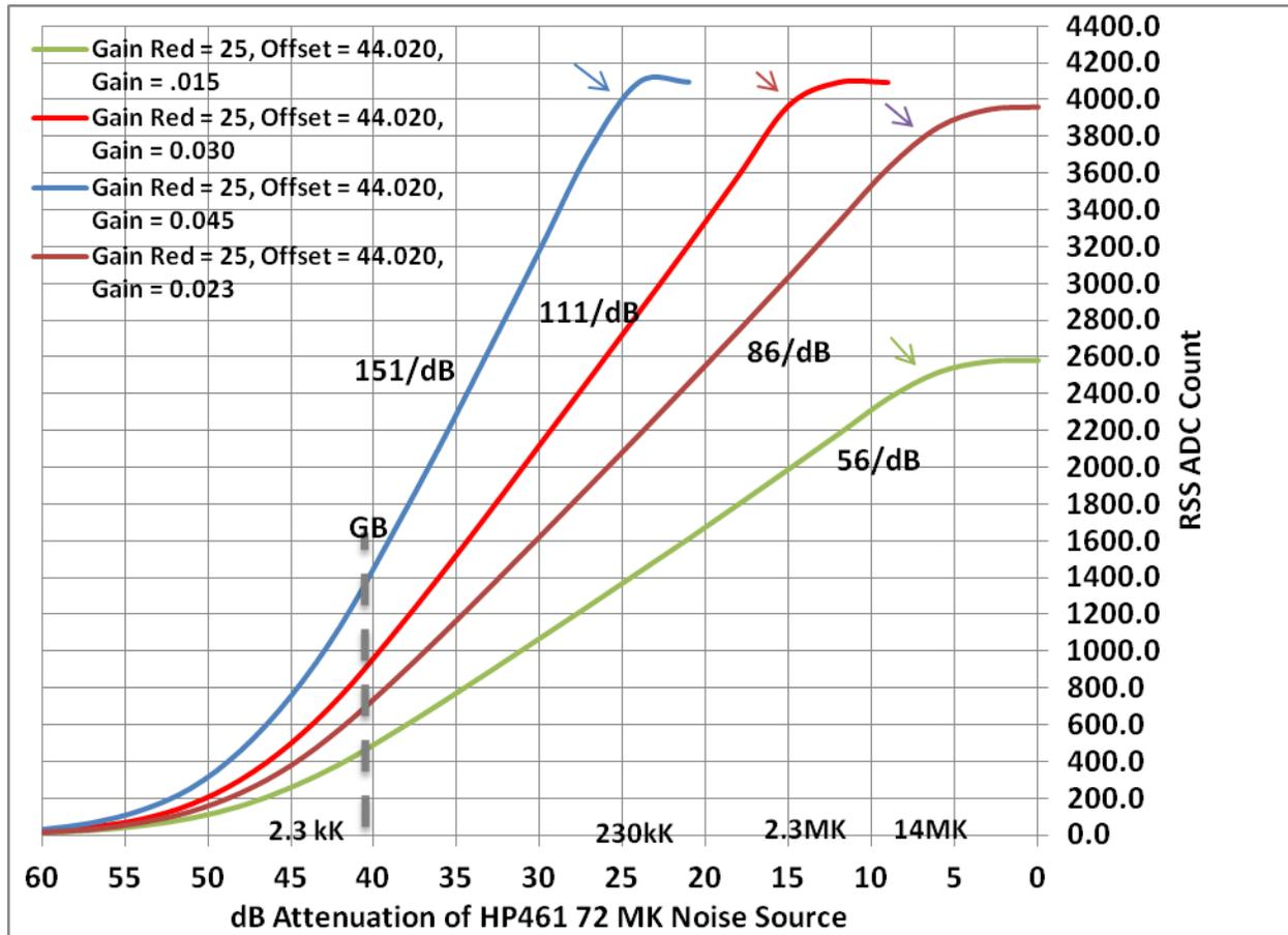
The horizontal axis shows dB attenuation of the 72 MK source and also equivalent temperature values. For example the attenuation of 45 dB is equivalent to 2.3kK, while 15 dB attenuation yields 2.3MK.
