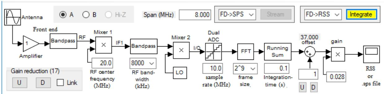
Figure 1 shows the settings for the RSP1-A from Nathan Towne’s SDRPlay2RSS interface and control panel used in this experiment.
