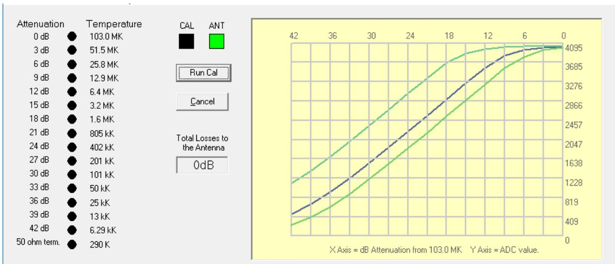
Figure 2 depicts the response curves of the RSP1-A with and without the multicoupler. The vertical axis of the plot represents the ADC count (signal strength) and the horizontal axis is input temperature given in dB of attenuation of a 103 kK noise generator. The left hand column of Figure 2 gives the relationship between attenuation and input temperature.
