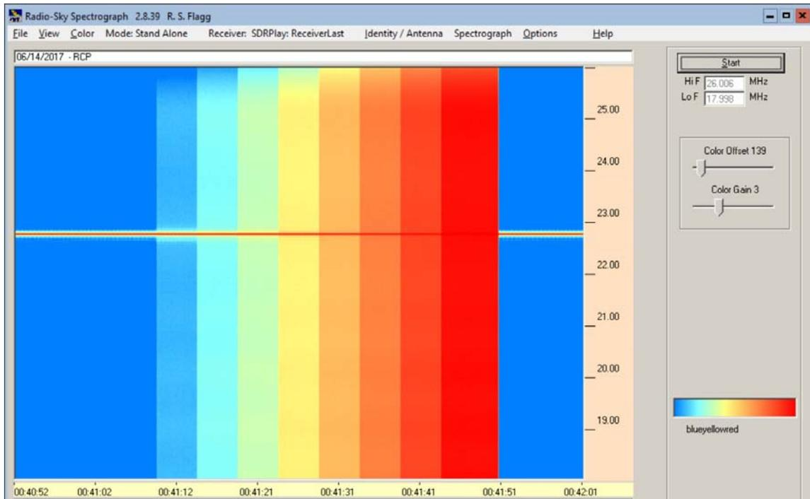
Fast Jupiter Cal on Radio Sky Spectrograph using an SDRPlay2
