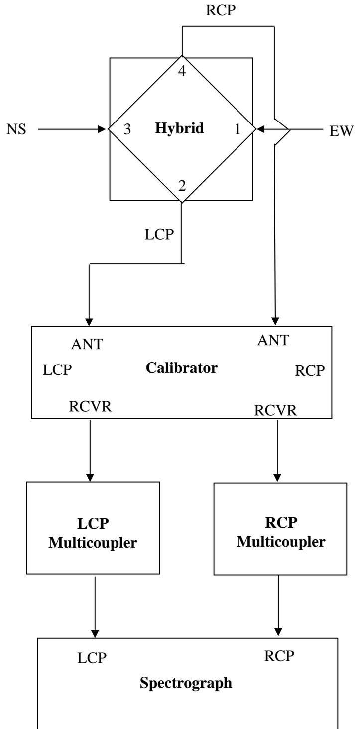
**Receiving System RF Connections for Hybrid after the Calibrator**
