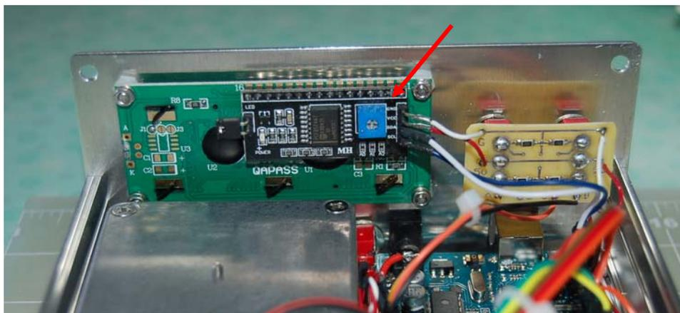
Blue trimpot intensity control on the rear of the display board.
