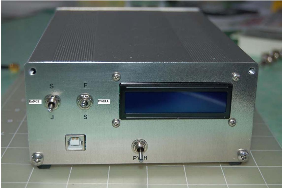
The **dwell time** is controlled by a two position toggle switch labeled **F** (for Fast) and **S** (for slow). The fast cal dwell time is 5 seconds per step and the slow dwell time is 10 seconds per step. Set the desired dwell time before initiating the cal run with the range switch..
