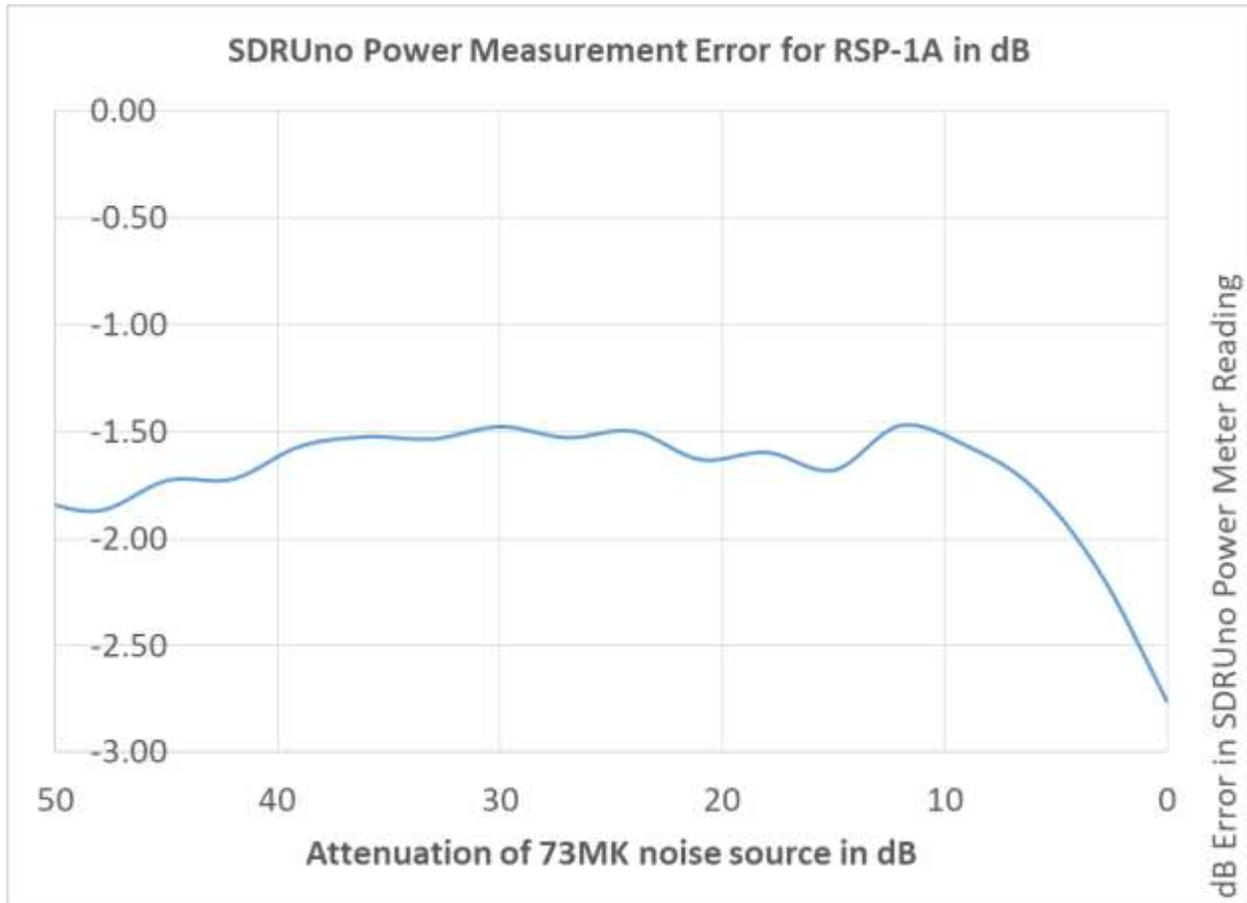
Figure 2 The vertical scale is measurement error in dB and the horizontal axis should be in 5 dB increments (Microsoft Excel refuses to do what I ask it to do).
