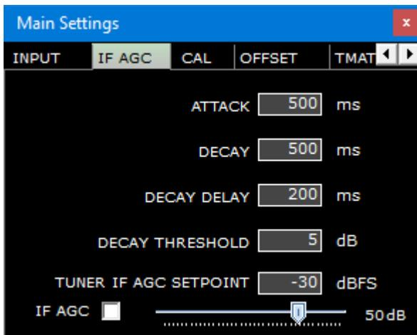
Figure 4 AGC OFF – manual gain
