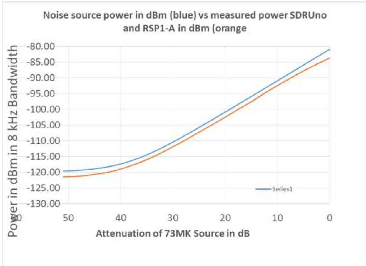
Figure 1 The input power to the RSP1-A in dBm is shown by the blue line. The input power level reported by SDRUno is shown by the orange line.
